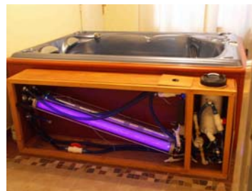
pilot photoreactor for spa water purification
