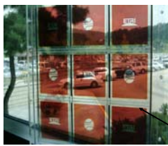
dye-sensitized solar cell in window panel
